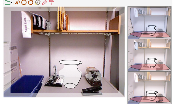
Figure 3. Our user interface consists of two main panels: a sketching panel where the user sketches on top of an RGB-D image to create s-canvas and a candidate panel where best-ranked candidate s-canvas are listed. The red and blue polygons are the supporting planes for the profile and trajectory strokes, respectively.
