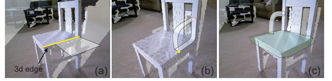
Figure 9. Various snapping cases enabled in our system: (a) snap to edge, (b) snap to point, and (c) snap to face.
